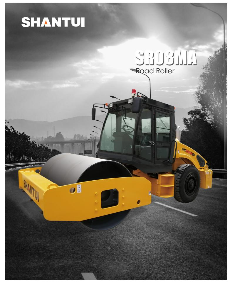
Engine Model: Gross Power: Operating Weight: Xinchai A498BG 42kW @2200rpm 8,000kg Focus on soil compaction road construction expert
